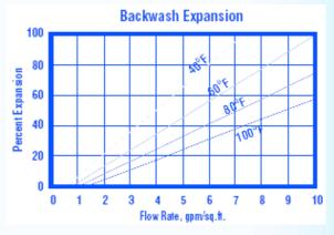
**Backwash:** After each cycle the resin bed should be backwashed at a rate that expands the bed 50 to 75 percent. This will remove any foreign matter and reclassify the bed. The graph above shows the expansion characteristics of Pure PC002 in the sodium form.
